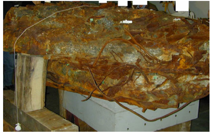
Figure 8: The reddish (rust) color of similar, previously-molten, Ground Zero debris, shown in this warehouse photo, indicates the presence of iron or steel.
