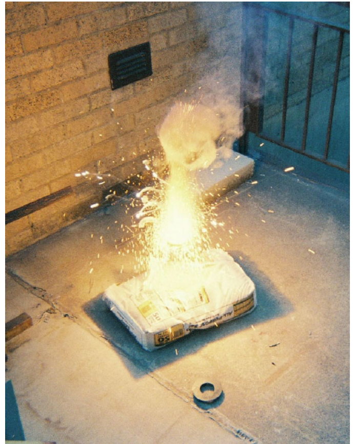
Figure 3: A thermite reaction generates yellow-white hot molten iron at well over 2,500°C/4,000°F and white smoke. This type of material can melt and cut steel beams.
