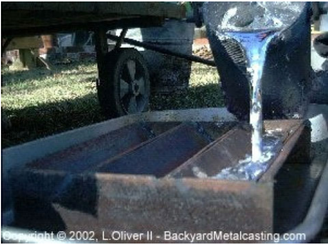
Figure 4: Molten aluminum appears silvery when poured in daylight conditions, even if initially heated to the yellow-white temperature range in the crucible.
